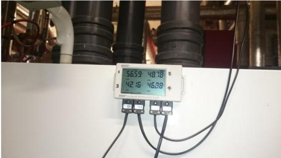
Using a four channel data logger enables us to track and analyse the performance of each circuit and make comparisons with the boiler set-points
